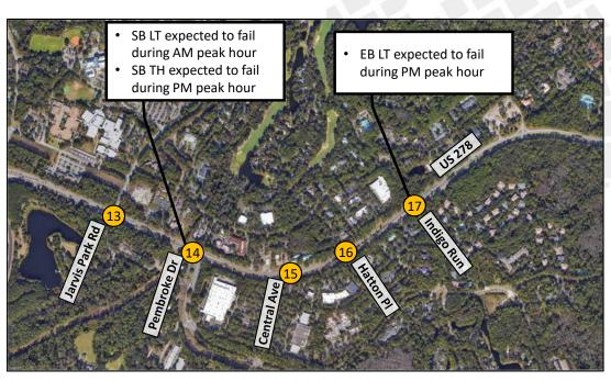
Even with the adaptive signals and reconfiguration of the northbound approach at Pembroke Dr to allow more of the cycle length to go to the mainline, long queues would still be expected between Gumtree Rd and Pembroke Ave. However, it is not expected that the maximum queue would extend into nearby intersections.
