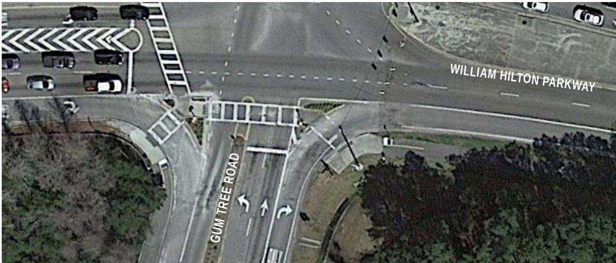
Slip lanes create multiple pedestrian conflict points and typically result in large turning radii. Removing slip lanes from intersections will create safer pedestrian crossings, minimizing high speed conflict points with vehicles.
