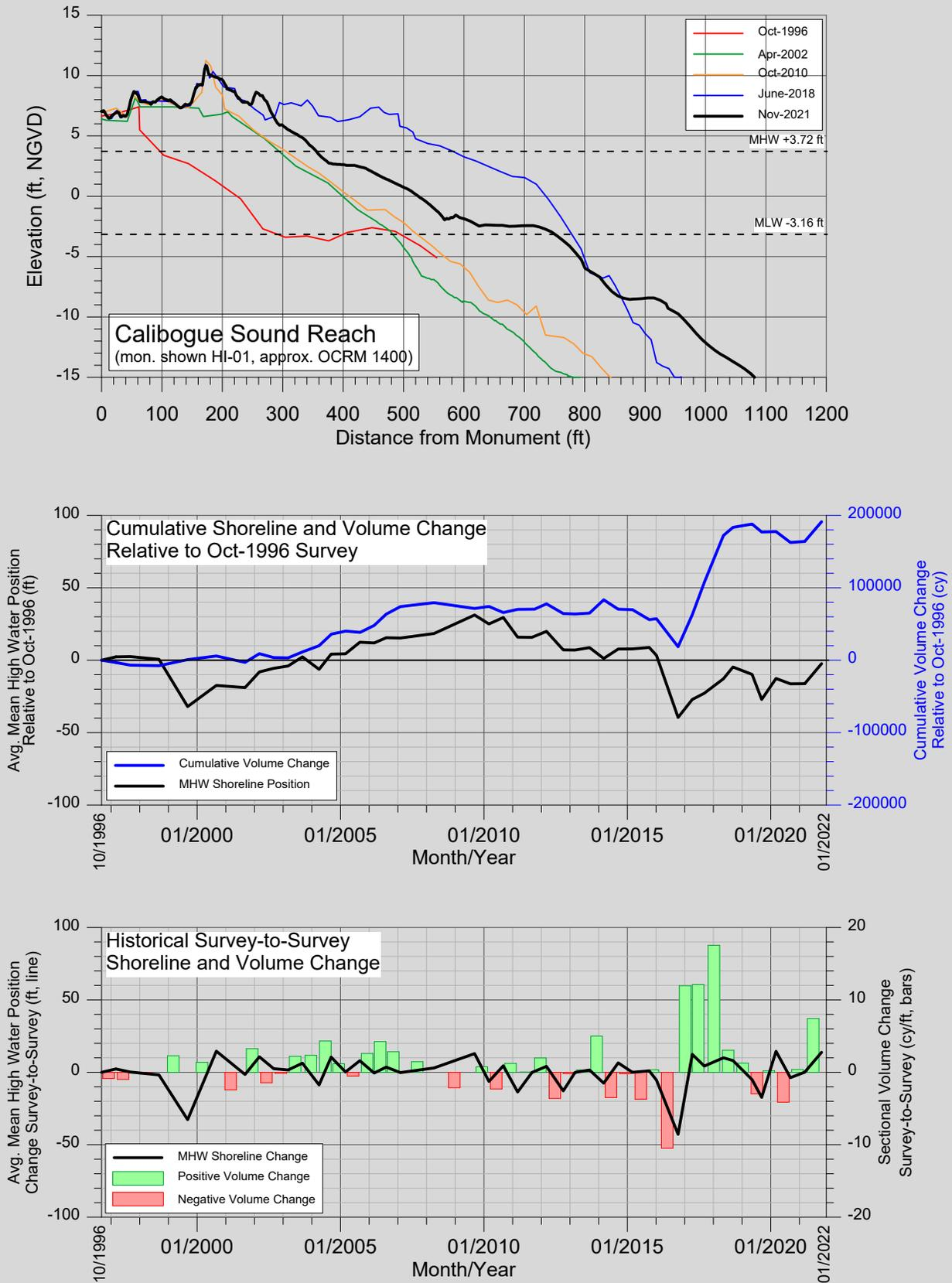
Figure 18: Calibogue sound changes (Oct-1994 to Nov-2021).
