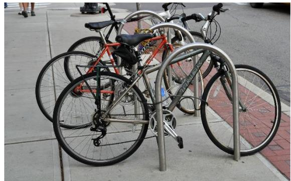
Inverted-U bicycle rack. Photo credit: cyclesafe.com
