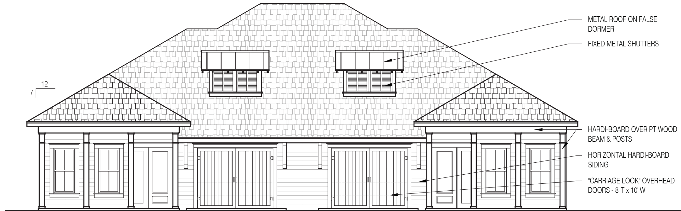
2 BUILDING C FRONT ELEVATION SCALE: 1/8" = 1'-0"
