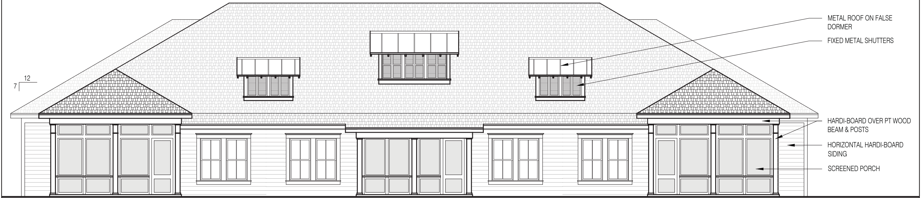
2 BUILDING D FRONT ELEVATION SCALE: 1/8" = 1'-0"
