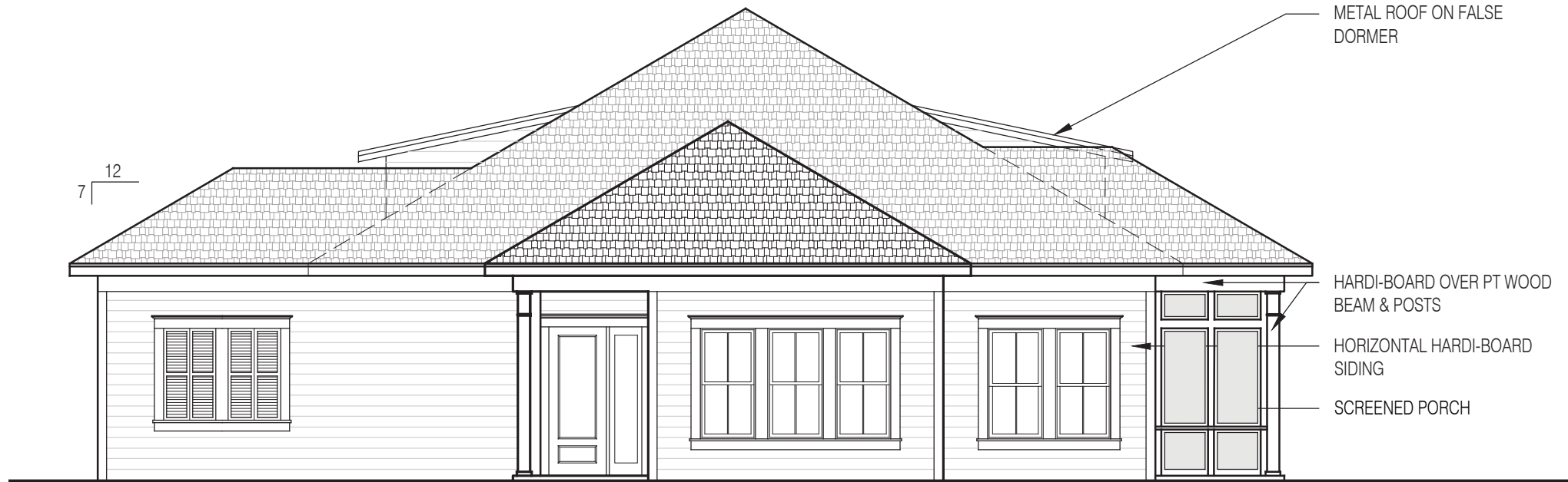
2 BUILDING A LEFT SIDE ELEVATION (ENTRY) SCALE: 1/8" = 1'-0"
