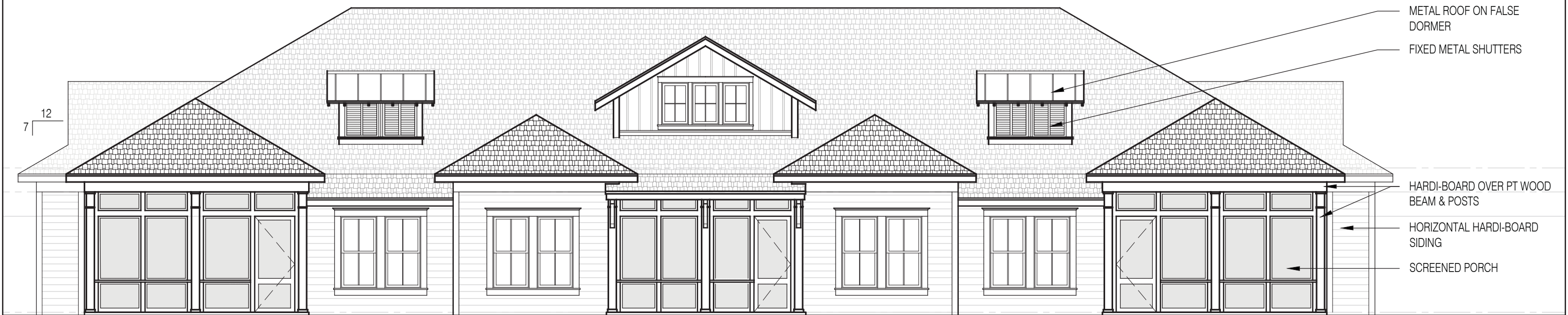
1 BUILDING B REAR ELEVATION SCALE: 1/8" = 1'-0"
