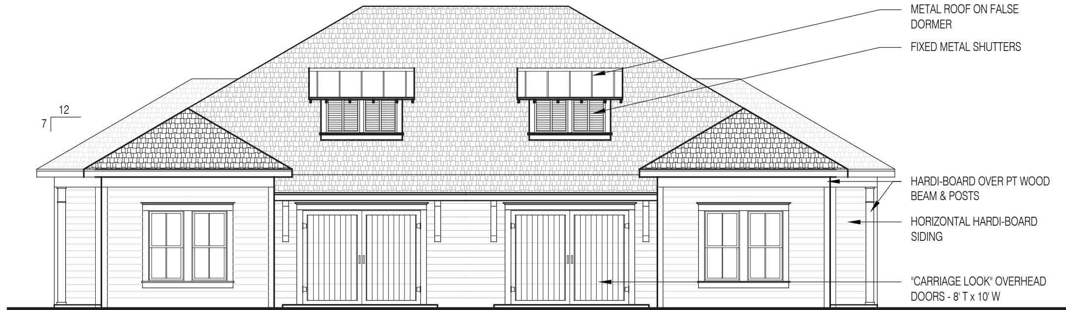
2 BUILDING A FRONT ELEVATION SCALE: 1/8" = 1'-0"
