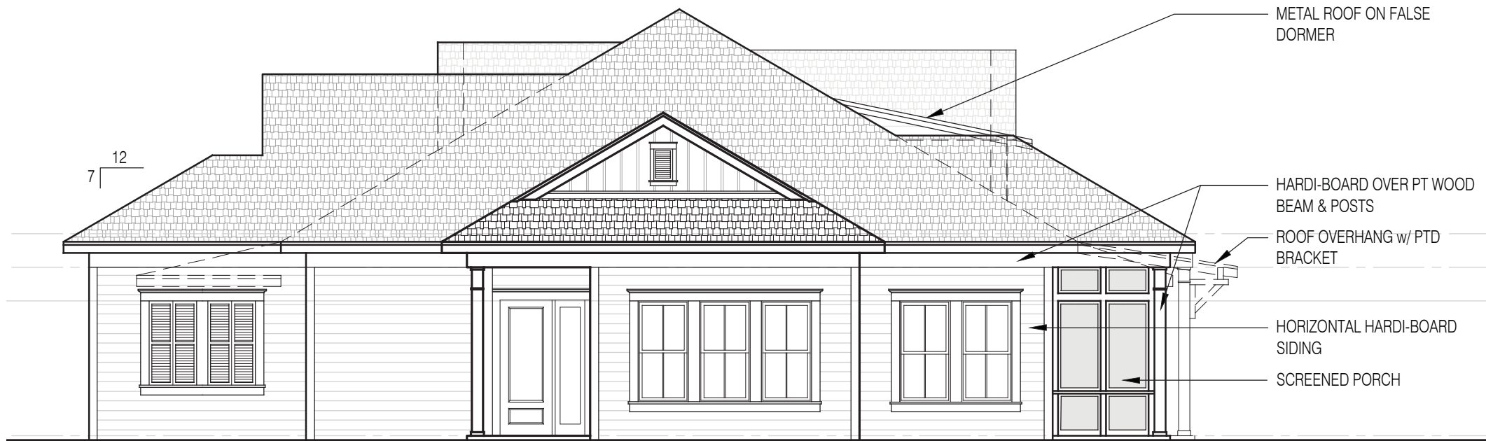
1 BUILDING B RIGHT SIDE ELEVATION (ENTRY) SCALE: 1/8" = 1'-0"
