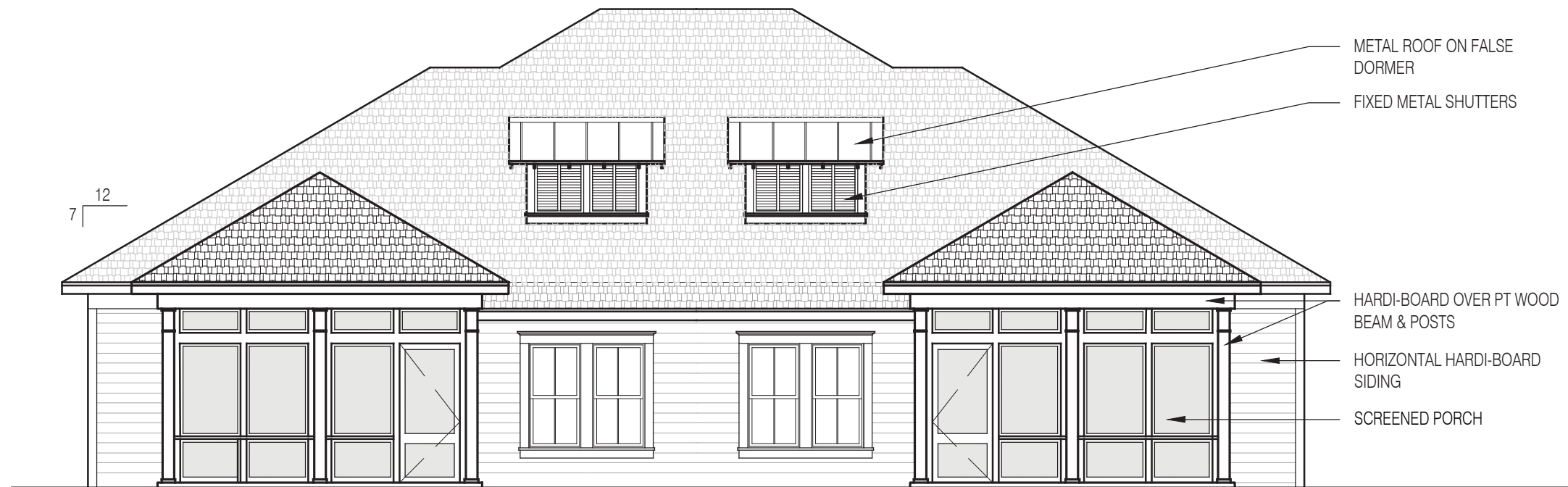
2 BUILDING C FRONT ELEVATION SCALE: 1/8" = 1'-0"
