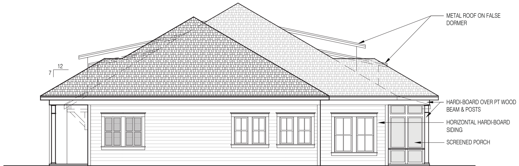
2 BUILDING D LEFT SIDE ELEVATION SCALE: 1/8" = 1'-0"
