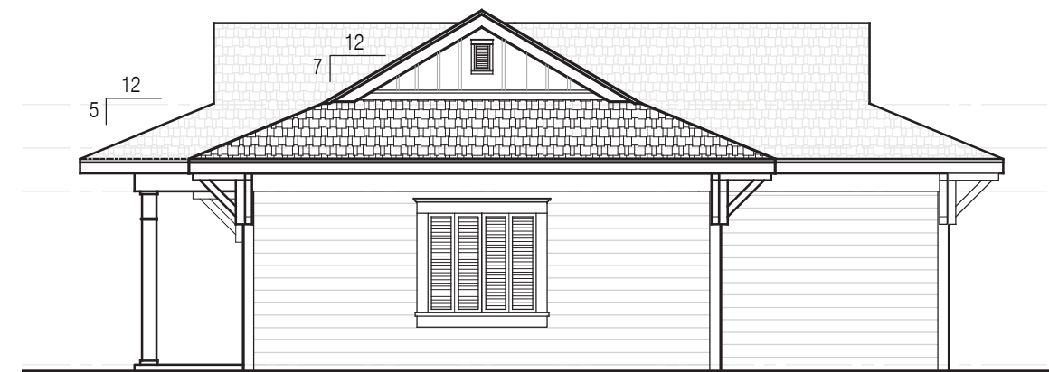
3 MAINTENANCE BUILDING RIGHT SIDE ELEVATION
