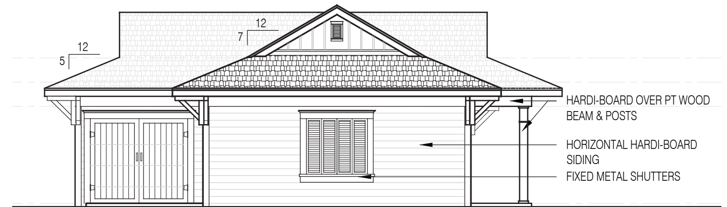
4 MAINTENANCE BUILDING LEFT SIDE ELEVATION
