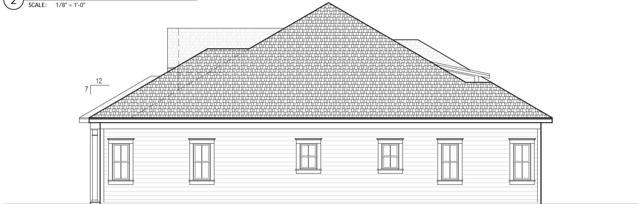
1 BUILDING E RIGHT SIDE ELEVATION SCALE: 1/8" = 1'-0"
