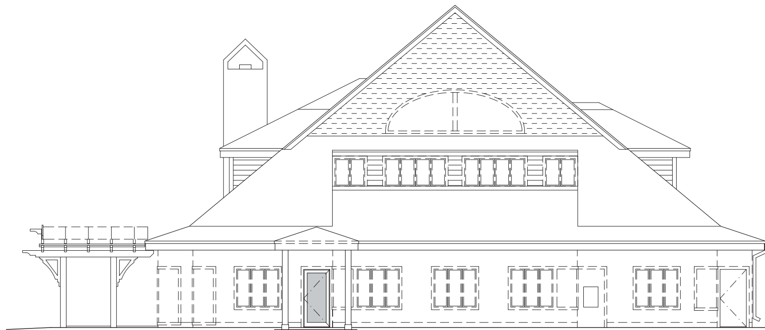
2 D3.0 SCALE 1/4" = 1'-0" NORTHEAST EXTERIOR DEMOLITION ELEVATION (RIGHT)
