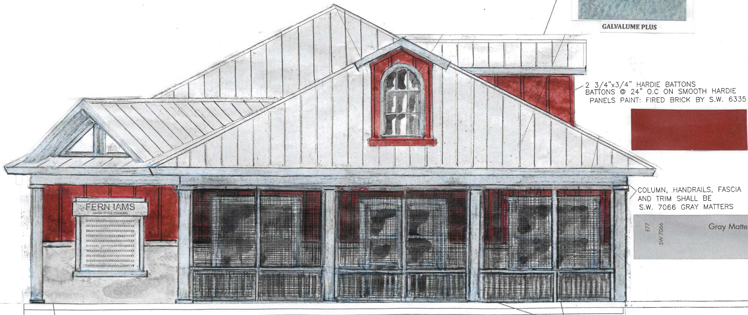
1"X2" EXTRUDED ALUMINUM SCREEN SYSTEM OVER RAILING ; PAINT GRAY MATTERS : S.W. 7056
