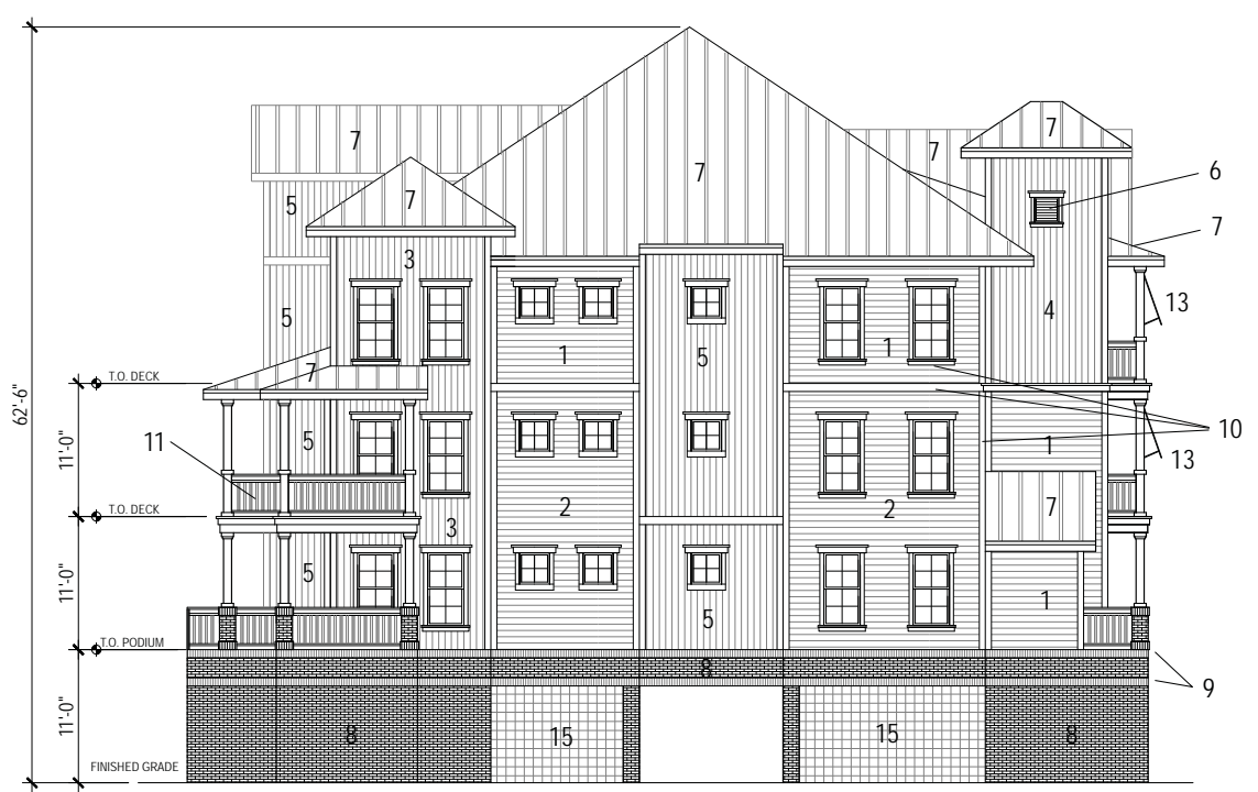
2 13 Unit Building- Left Elevation SCALE: 1/8" = 1'-0"
