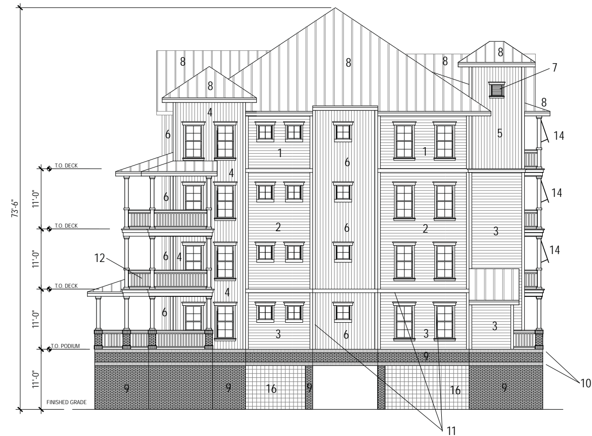
2 30 Unit Building- Left Elevation SCALE: 1/8" = 1'-0"
