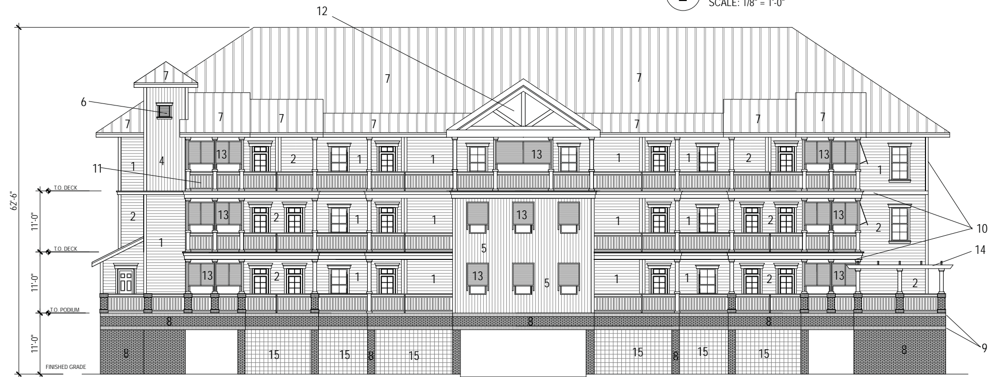
1 16 Unit Building- Front Elevation SCALE: 1/8" = 1'-0"
