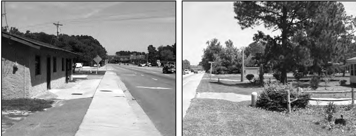
Figure 17: Illustration of setbacks. The photo on the left shows a building with no setback from the street right-of-way, while the photo on the right shows a building with a substantial setback.
