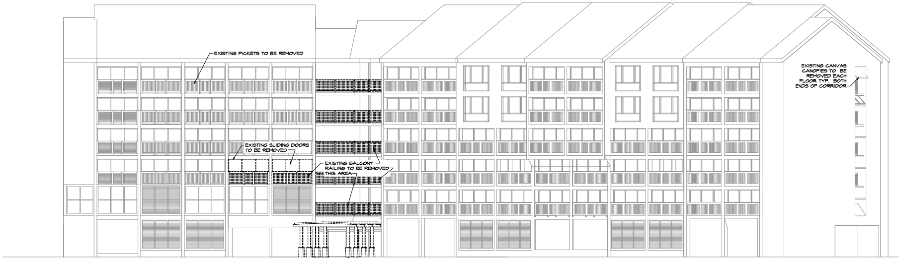
1 FRONT ENTRY DEMO ELEVATION 1/8" = 1'-0"
