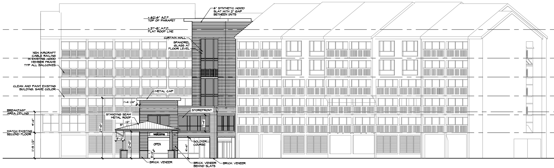
2 FRONT ENTRY ELEVATION 1/8" = 1'-0"
