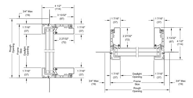
Direct Glaze Rectangle Head Jamb and Sill with 1 1/4" Triple-Pane Direct Glaze Rectangle Jambs with 1 1/4" Triple-Pane
