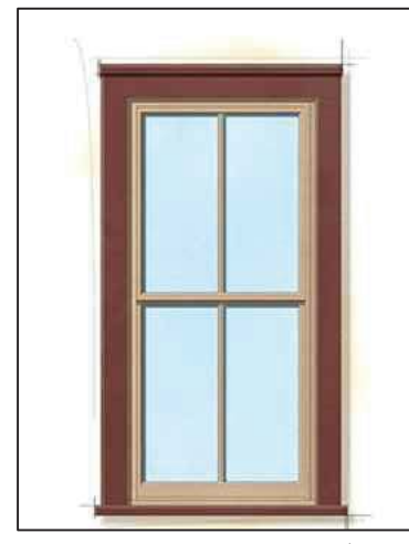
SINGLE HUNG WINDOW UNIT (2 OVER 2) MANUFACTURER: JELDWEN PREMIUM ATLANTIC VINYL COLOR: WHITE
