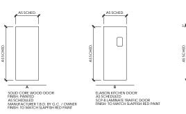
A H.M. FRAME (PAINTED) AS SCHEDULED MANUFACTURER T.B.D. BY G.C. / OWNER NON-FERROUS AT EXTERIOR OPENINGS
