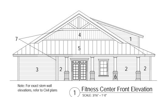
1-Hardie Lap Siding- Sandstone Beige 2-Hardie Lap Siding- Heathered Moss 3-Hardie Lap Siding- Mountain Sage 4-Hardie Vertical Siding- Sandstone Beige
