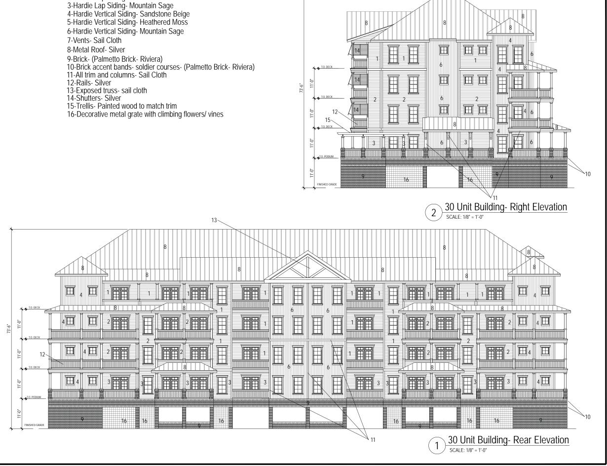
1-Hardie Lap Siding- Sandstone Beige 2-Hardie Lap Siding- Heathered Moss
