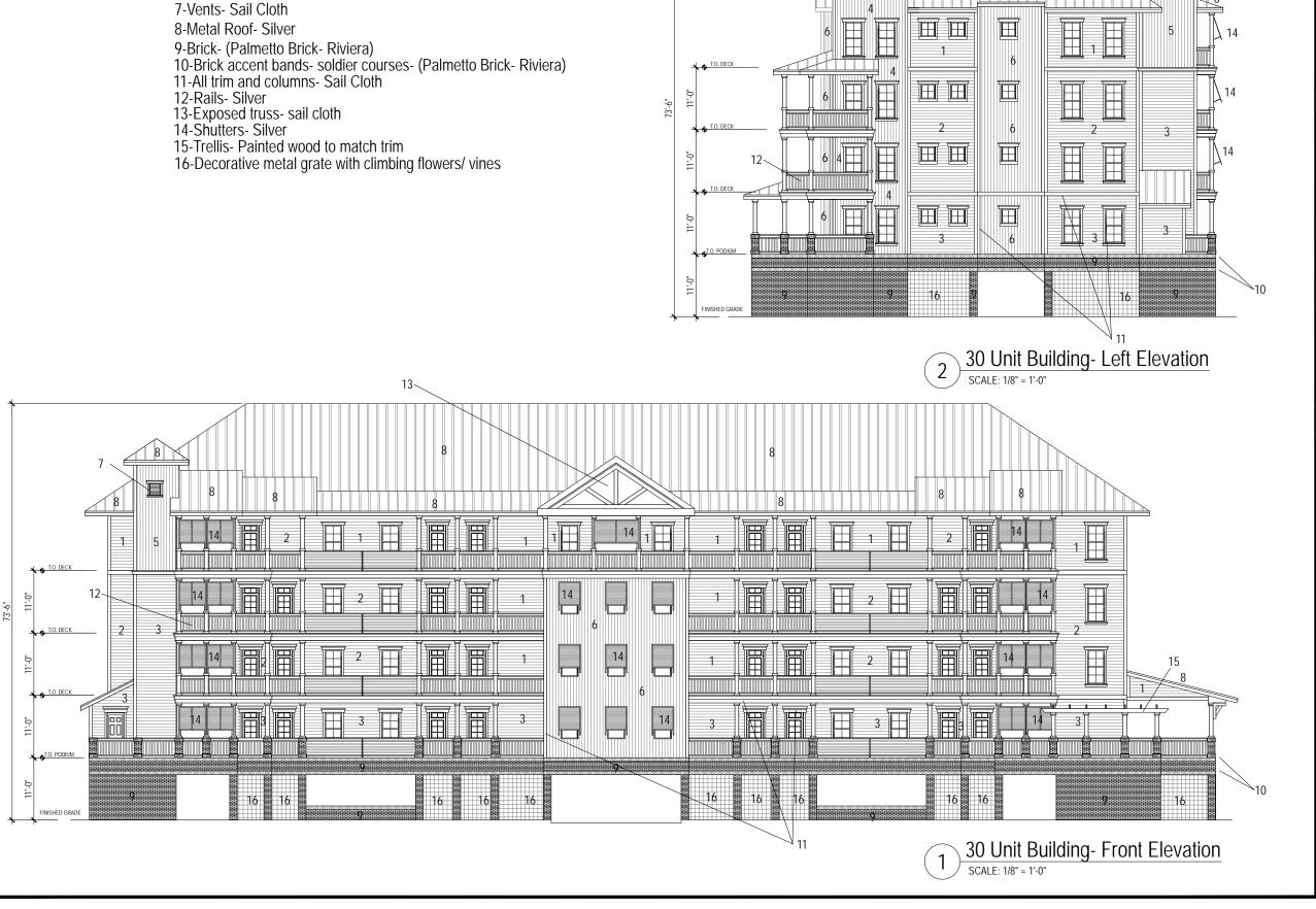
1-Hardie Lap Siding- Sandstone Beige 2-Hardie Lap Siding- Heathered Moss 3-Hardie Lap Siding- Mountain Sage 4-Hardie Vertical Siding- Sandstone Beige 5-Hardie Vertical Siding- Heathered Moss 6-Hardie Vertical Siding- Mountain Sage
